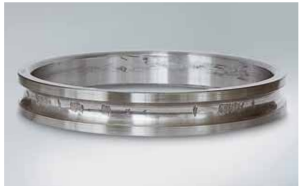
Photo 1.4 Part: Inner ring of an angular contact ball bearing Symptom: Flaking of raceway at ball pitch Cause: Dents due to shock load while stationary
