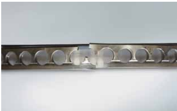
Photo 7.3 Part: Cage of an angular contact ball bearing Symptom: Fracture of machined high-tension brass cage
