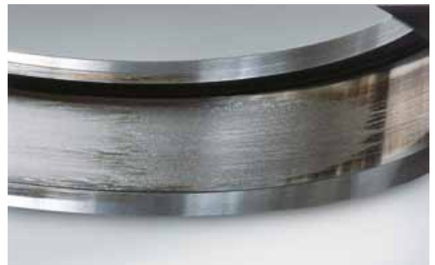
Photo 4.2 Part: Outer ring of Photo 7-4-1 Symptom: Smearing occurs circumferentially on raceway surface Cause: Roller slipping due to excessive grease filling
