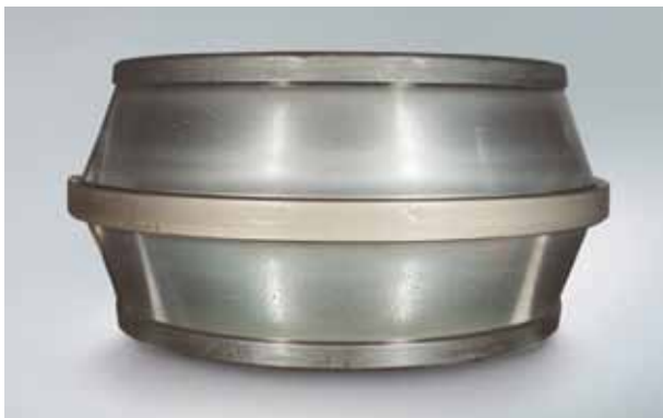
Photo 8.1 Part: Inner ring of a double-row tapered roller bearing Symptom: Frosted raceway surface Cause: Debris caught in the surface
