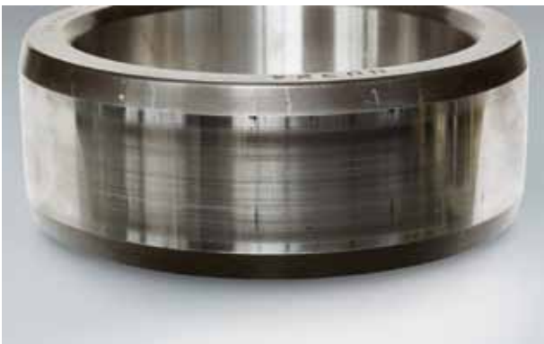
Photo 17.1 Part: Inner ring of a cylindrical roller bearing Symptom: Axial scratches on raceway surface Cause: Inclination of inner and outer rings during mounting
