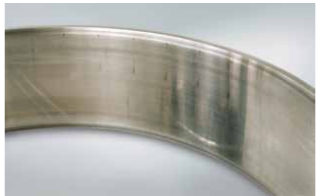
Photo 17.2 Part: Outer ring of a double-row cylindrical roller bearing Symptom: Axial scratches at roller pitch intervals on raceway surface Cause: Inclination of inner and outer rings during mounting
