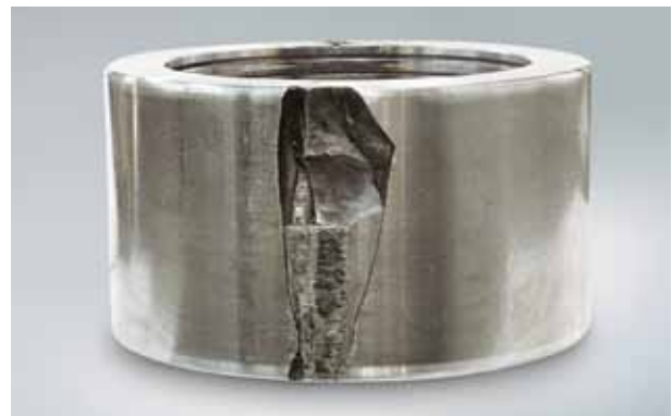
Photo 6.4 Part: Outer ring of a double-row cylindrical roller bearing used for outer ring rolling (Outer ring rotation) Symptom: Cracks occur on outside surface Cause: Flat wear and heat generation due to non-rotation of the outer ring
