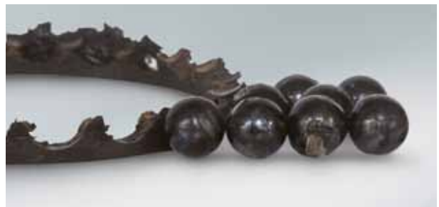
Photo 14.5 Part: Balls and cage of Photo 7-14-3 Symptom: Cage is damaged by melting, balls become discolored and melted Cause: Excessive preload
