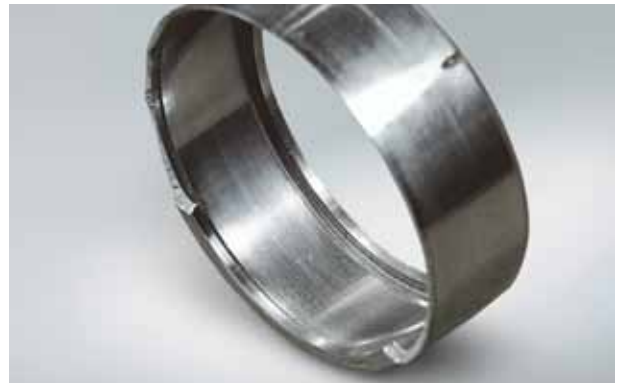
Photo 5.4 Part: Outer ring of a solid type needle roller bearing Symptom: Fracture occurs at the outer ring rib Cause: Roller inclination due to excessive loading (Needle rollers are long compared to their diameter. Under excessive or uneven loading, rollers become inclined and push against the ribs.)
