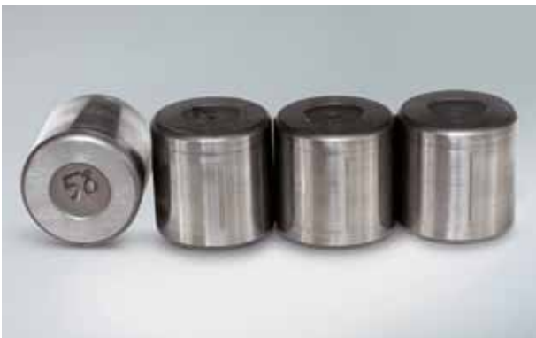
Photo 17.3 Part: Rollers of a cylindrical roller bearing Symptom: Axial scratches on rolling surface Cause: Inclination of inner and outer rings during mounting
