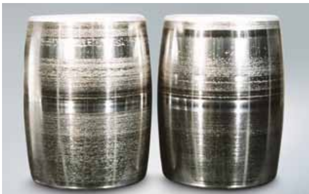
Photo 4.7 Part: Convex rollers of Photo 7-4-5 Symptom: Smearing occurs at the center of the rolling surface Cause: Poor lubrication
