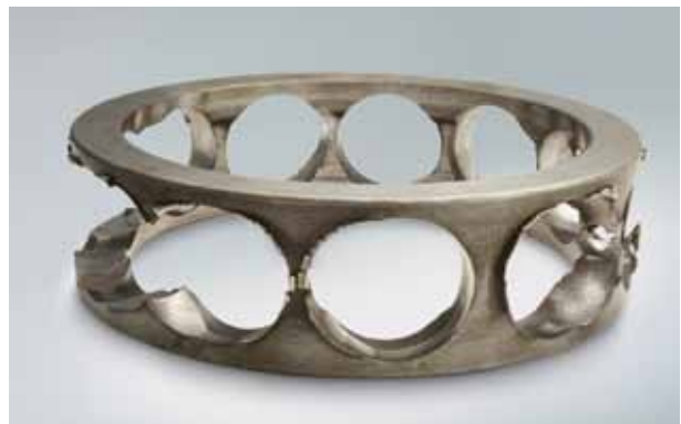
Photo 7.2 Part: Cage of an angular contact ball bearing Symptom: Pocket pillar fractures from a cast iron machined cage Cause: Abnormal load action on cage due to misaligned mounting between inner and outer rings
