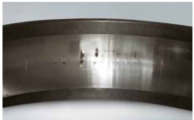
Photo 12.2 Part: Outer ring of Photo 7-12-1 Symptom: False brinelling occurs on the raceway Cause: Vibration from an external source while stationary
