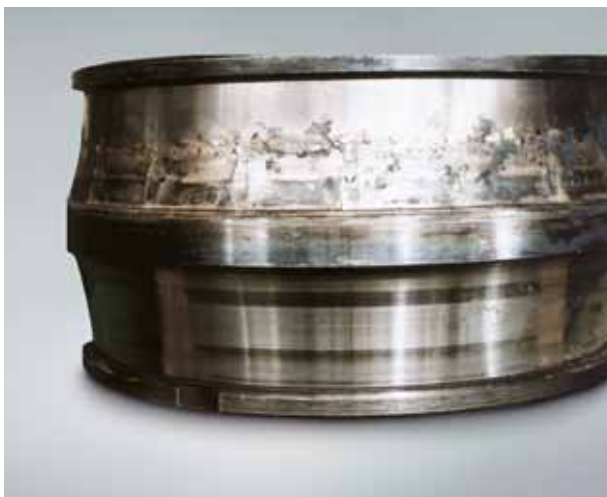
Photo 14.1 Part: Inner ring of a spherical roller bearing Symptom: Raceway is discolored and melted. Worn particles from the cage were rolled and attached to the raceway Cause: Insufficient lubrication
