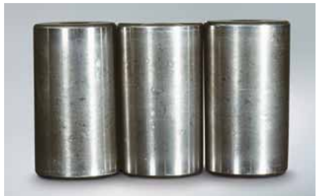
Photo 8.4 Part: Tapered rollers of Photo 7-8-3 Symptom: Small and large indentations occur over the rolling surface Cause: Debris caught in the surface
