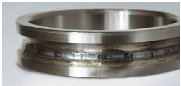
Photo 14.3 Part: Inner ring of an angular contact ball bearing Symptom: Raceway discoloration, melting occurs at ball pitch intervals Cause: Excessive preload
