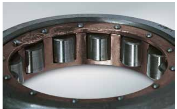
Photo 7.6 Part: Cage of a cylindrical roller bearing Symptom: Deformation of the side face of a machined high-tension brass cage Cause: Large shock during mounting
