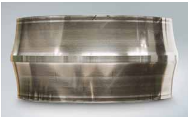
Photo 4.3 Part: Inner ring of a spherical roller bearing Symptom: Smearing occurs circumferentially on raceway surface Cause: Poor lubrication
