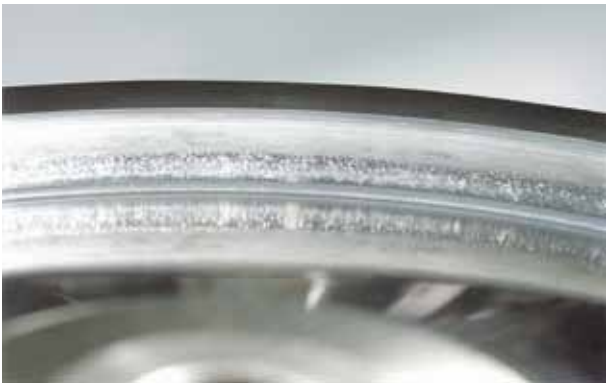
Photo 3.3 Part: Inner ring of a tapered roller thrust bearing Symptom: Scoring on the face of inner ring rib Cause: Worn particles become mixed with lubricant, and breakdown of oil film occurs due to excessive load
