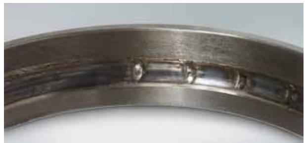
Photo 14.4 Part: Outer ring in Photo 7-14-3 Symptom: Raceway discoloration, melting occurs at ball pitch intervals Cause: Excessive preload
