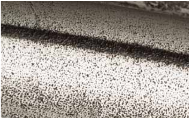
Photo 9.1 Part: Outer ring of a slewing bearing Symptom: Pitting occurs on the raceway surface Cause: Rust at bottoms of indentations
