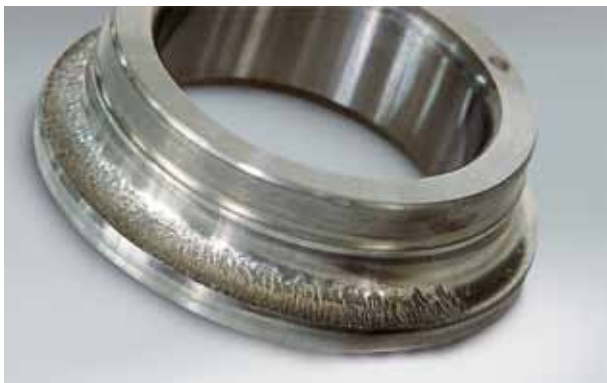
Photo 1.1 Part: Inner ring of an angular contact ball bearing Symptom: Flaking occurs around half of the circumference of the raceway surface Cause: Poor lubrication due to entry of cutting coolant into bearing
