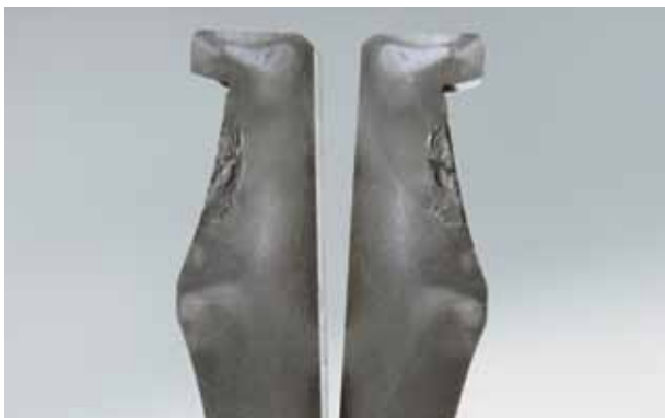
Photo 6.7 Part: Cross section of a fractured inner ring in Photo 7-6-6 Symptom: Origin is directly beneath the raceway surface
