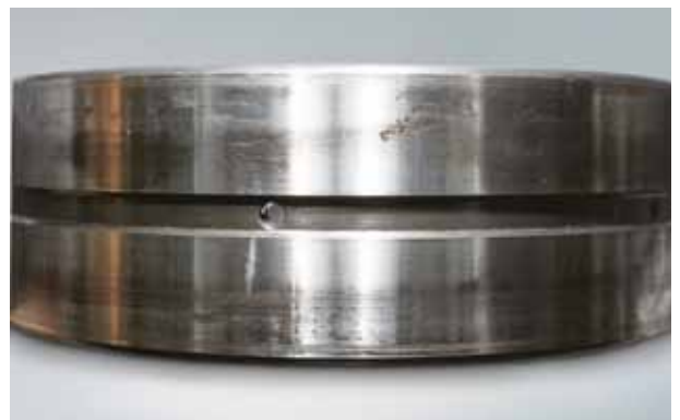
Photo 13.2 Part: Outer ring of a spherical roller bearing Symptom: Creep occurs over entire circumference of outside surface Cause: Loose fit between outer ring and housing
