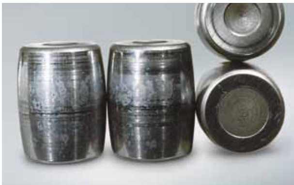
Photo 2.3 Part: Convex rollers of Photo 7-2-1 Symptom: Round shaped peeling pattern occurs on the center of the rolling surfaces Cause: Poor lubrication
