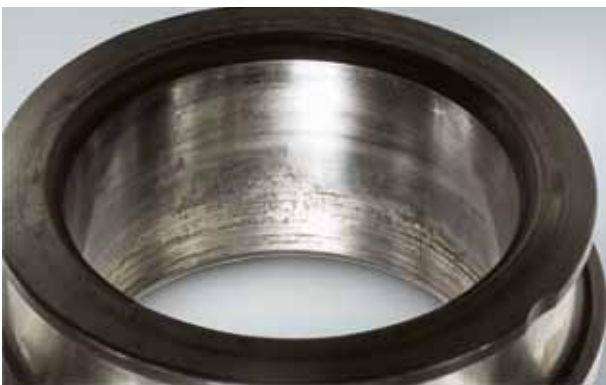
Photo 13.1 Part: Inner ring of a spherical roller bearing Symptom: Creep accompanied by scoring of bore surface Cause: Insufficient interference
