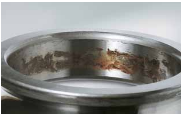
Photo 11.1 Part: Inner ring of a deep groove ball bearing Symptom: Fretting occurs on the bore surface Cause: Vibration
