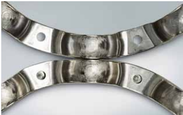
Photo 3.7 Part: Cage of a deep groove ball bearing Symptom: Scoring on the pressed-steel cage pockets Cause: Entry of debris
