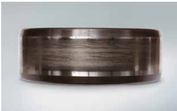
Photo 4.1 Part: Inner ring of a cylindrical roller bearing Symptom: Smearing occurs circumferentially on raceway surface Cause: Roller slipping due to excessive grease filling
