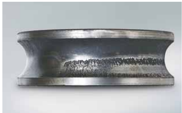
Photo 1.2 Part: Inner ring of an angular contact ball bearing Symptom: Flaking occurs diagonally along raceway Cause: Poor alignment between shaft and housing during mounting
