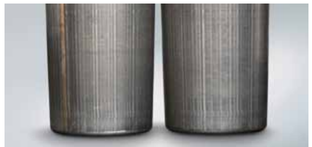
Photo 15.2 Part: Tapered rollers in Photo 7-15-1 Symptom: Striped pattern of corrosion occurs on the rolling surface
