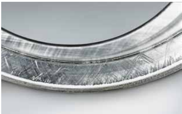
Photo 3.5 Part: Inner ring of a spherical thrust roller bearing Symptom: Scoring on the rib face of inner ring Cause: Debris, which is caught in surface, and excessive axial loading
