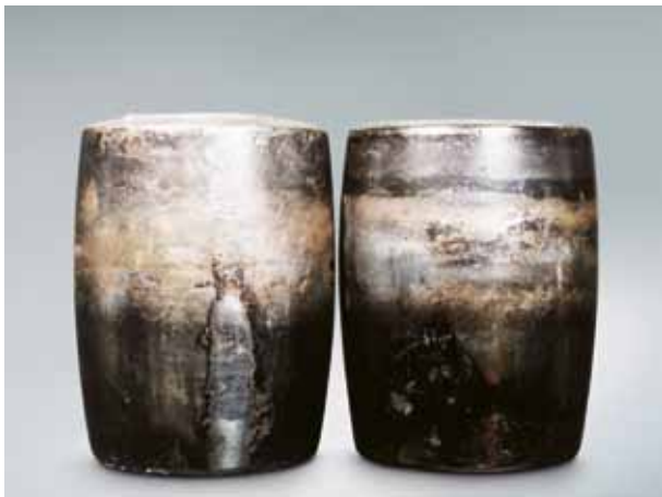
Photo 14.2 Part: Convex rollers of Photo 7-14-1 Symptom: Discoloration and melting of roller rolling surface, adhesion of worn particles from cage Cause: Insufficient lubrication
