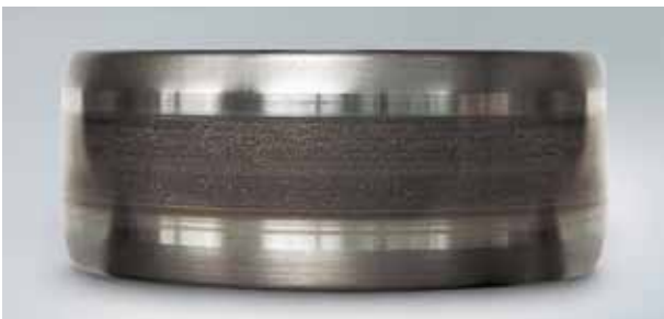
Photo 15.3 Part: Inner ring of a cylindrical roller bearing Symptom: Belt pattern of electrical corrosion accompanied by pits on the raceway surface
