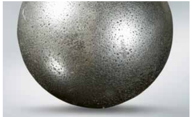
Photo 9.2 Part: Ball of Photo 7-9-1 Symptom: Pitting occurs on the rolling element surface
