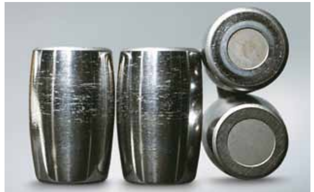
Photo 3.2 Part: Convex rollers of Photo 7-3-1 Symptom: Scoring on roller end face Cause: Roller slipping due to sudden acceleration and deceleration
