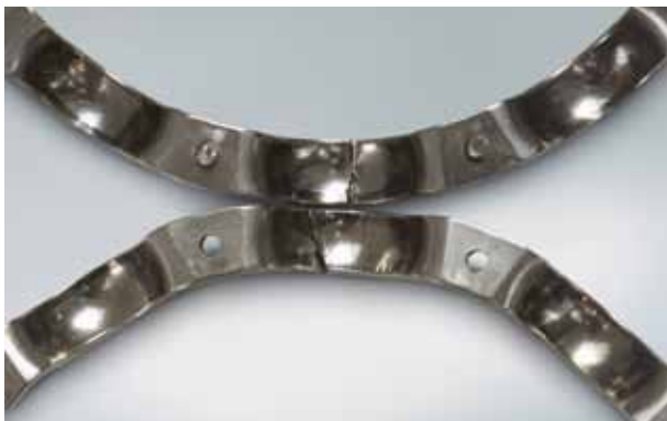
Photo 7.1 Part: Cage of a deep groove ball bearing Symptom: Fracture of pressed-steel cage-pocket
