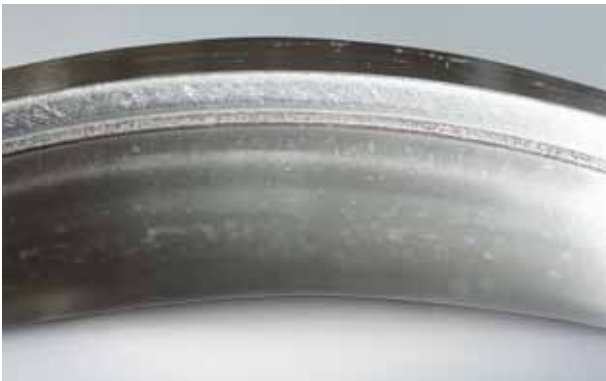
Photo 3.1 Part: Inner ring of a spherical roller bearing Symptom: Scoring on large rib face of inner ring Cause: Roller slipping due to sudden acceleration and deceleration
