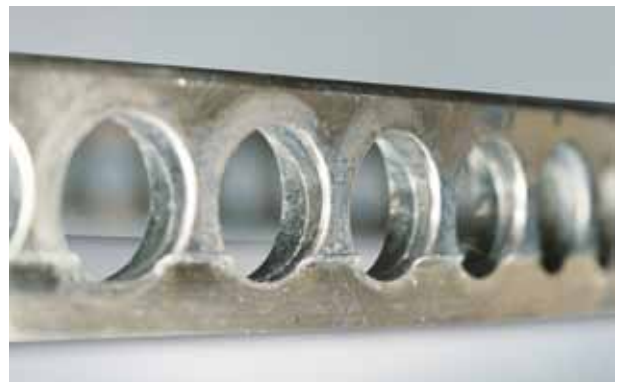
Photo 7.8 Part: Cage of an angular contact ball bearing Symptom: Stepped wear on the outside surface and pocket surface of a machined high-tension brass cage
