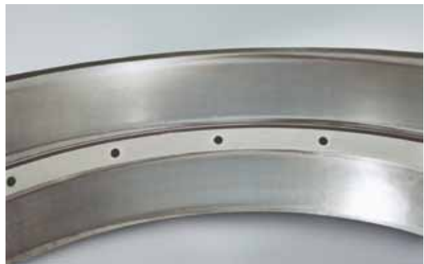
Photo 8.2 Part: Outer ring of a double-row tapered roller bearing Symptom: Indentations on raceway surface Cause: Debris caught in the surface
