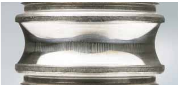
Photo 15.5 Part: Inner ring of a deep groove ball bearing Symptom: Fluting occurs on the raceway surface (High frequency)
