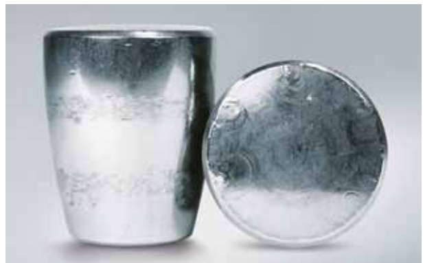
Photo 3.6 Part: Convex rollers of Photo 7-3-5 Symptom: Scoring on the roller end face Cause: Debris, which is caught in surface, and excessive axial loading
